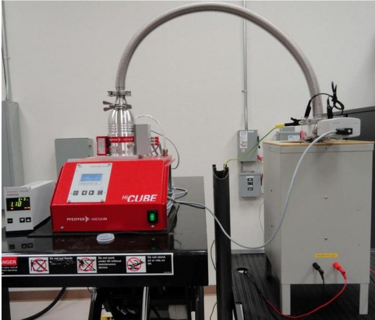
In order to create the ‘ionization current - pressure curve’ for the MAC-TS1 and MAC-TS2 Testers, 40 data points are required for each unique vacuum interrupter within the range  $1 \times 10^{-1}$  Pa -  $1 \times 10^{-5}$  Pa.
